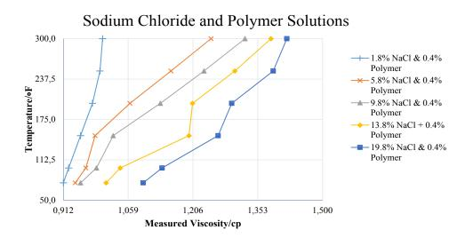
Fig. 8. Effect of temperature on viscosity the mixed of sodium chloride and polymer solutions.
