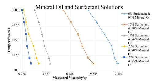
Fig. 7. Effect of temperature on viscosity the mixed of mineral oil and surfactant solutions.
