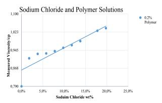
Fig. 6. Viscosity of the mixed of sodium chloride and polymer solutions.
