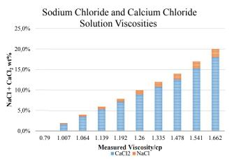
Fig. 5. Viscosity of the mixed of sodium chloride and calcium chloride solutions compared.
