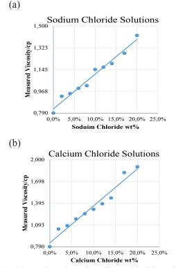
Fig. 4. (a) – viscosity of sodium chloride solutions; (b) – viscosity of calcium chloride solutions.
