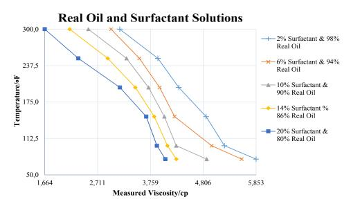
Fig. 9. Effect of temperature on viscosity of mixed real oil and surfactant solutions.
