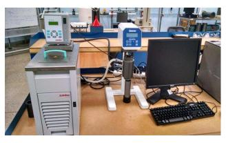
Fig. 3. Rheometer and Heat Bath Setup.
