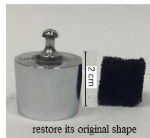
Fig. 4. Illustration of the compression process of PU sponge coated with MWCNTs with loading of 50 g followed by restoring its original shape.
