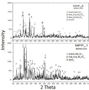
Fig. 2. X-ray powder diffractograms for Egyptian Blue, produced by SCS method at temperatures 700–850 °C.
