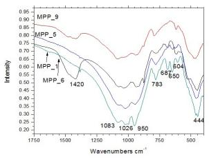
Fig. 5. IR spectra of Egyptian blue pigment prepared by SCS at different temperatures: MPP-1-850 °C, MPP-5-800 °C, MPP-9-750 °C, MPP-6-700 °C.
