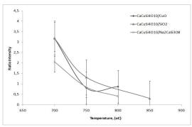
Fig. 3. The dependence of  $CaCuSi_4O_{10}/CuO$ ,  $CaCuSi_4O_{10}/SiO_2$  and  $CaCuSi_4O_{10}/Na_2CaSi_3O_8$  ratio from preheating temperature.
