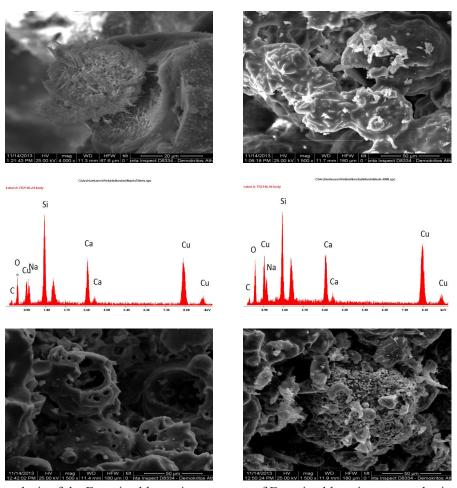
Fig. 4. SEM/EDX analysis of the Egyptian blue, microstructure of Egyptian blue pigment synthesized by SCS method.
