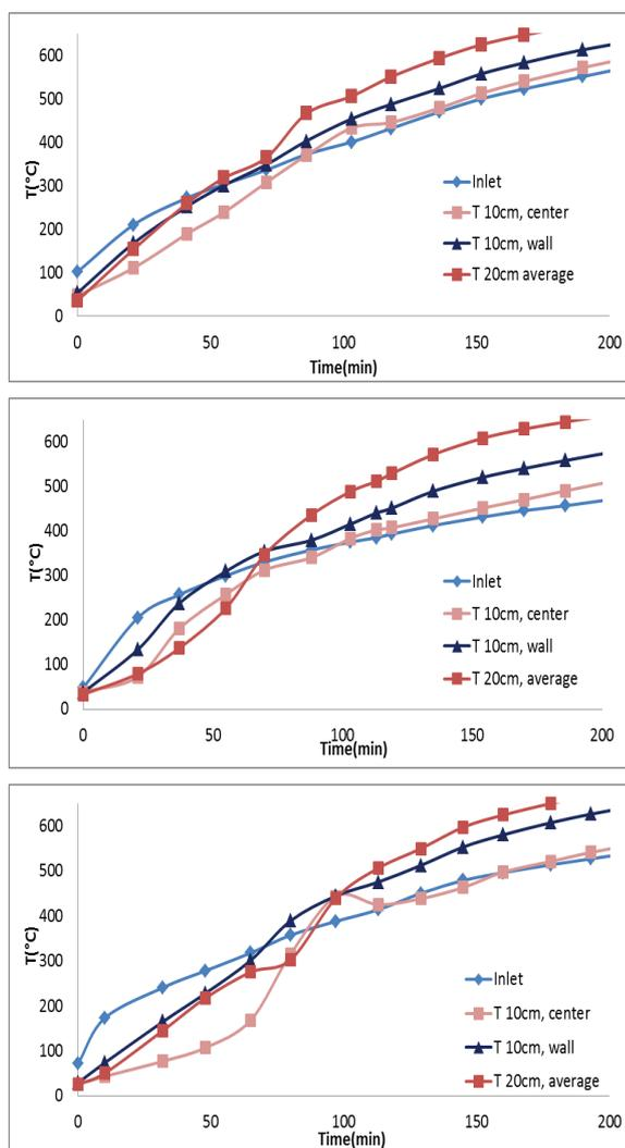
Fig. 2. Top – Comparison of temperatures evolution for wood chips with  $N_2$  flow rates of 20 l/min. Middle – Comparison of temperatures evolution for pine wood chips with  $N_2$  flow rates of 40 l/min. Bottom – Comparison of temperatures evolution for beech wood with  $N_2$  flow rates of 20 l/min.
