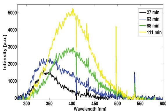
Fig. 12. Evolution of the fluorescence spectra during a gasification process.
