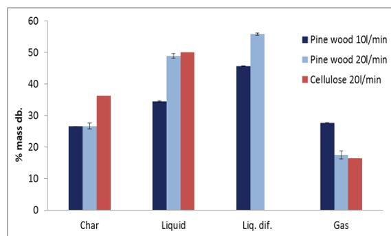
Fig. 4. Char, liquid, and gas yields of pyrolysis experiments. Liq. dif. corresponds to the liquid yield obtained by difference 100 – (% char + % gas).
