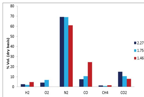
Fig. 10. Product gas composition of gasification process using three different air to fuel ratios in kg.
