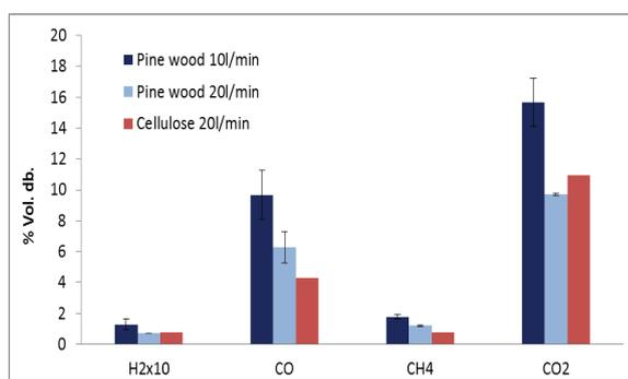
Fig. 5. Permanent gas composition for the experiments presented in Fig. 4.
