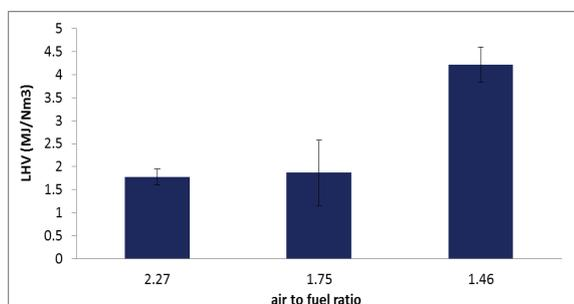
Fig. 11. Low heating value of the product gas for the three different process conditions presented in Fig. 10.
