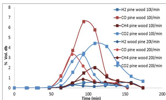
Fig. 6. Permanent gas evolution for the pyrolysis experiments of pine wood with 10 and 20 l/min.
