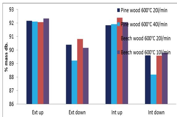
Fig. 9. Carbon content in mass percentage in dry basis for pine and beech pyrolysis up to a maximum temperature of 600 °C measured in the reference position and with flow rates of 10, 20, and 40 l/min.
