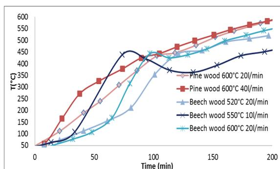
Fig. 3. Comparison of temperatures evolution in the reference position for several pyrolysis experiments.
