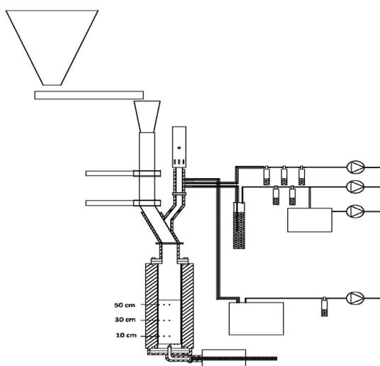
Fig. 1. Reactor set up: 1 – hopper, 2 – conveyor belt, 3 – feeding valves, 4 – burner, 5 – tar condensation line, 6 – GC-TCD, 7 – LIF system, 8 – Preheater.
