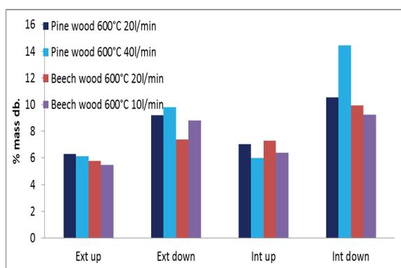
Fig. 8. Volatiles content in mass percentage in dry basis for pine and beech pyrolysis up to a maximum temperature of 600 °C measured in the reference position and with flow rates of 10, 20, and 40 l/min.
