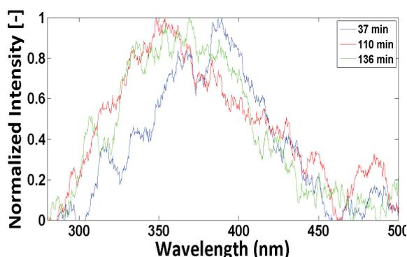
Fig. 7. Fluorescence spectra at different times from pine wood pyrolysis with a flow rate of 20 l/min [17].
