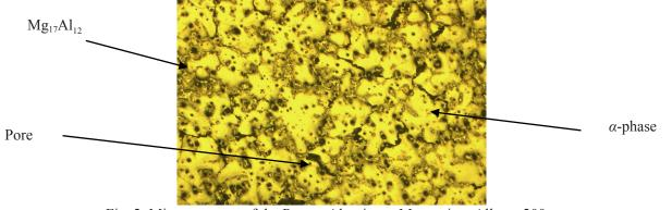
Fig. 2. Microstructure of the Porous Aluminum-Magnesium Alloy, x200.
