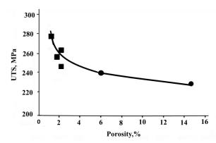
Fig. 3. Relationship between Tensile Strength and Porosity of Magnesium Alloys: ML5 (AZ91E), where  $\blacksquare$  – under the data from [6, 12],  $\bullet$  – under the authors' data.
