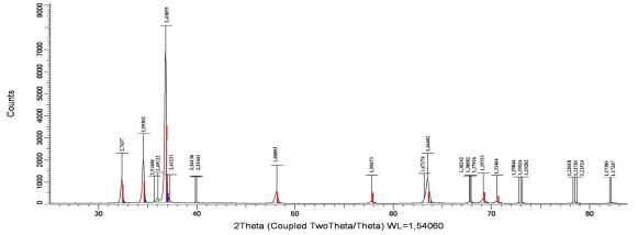
Fig. 1. X-Ray Analysis of the Porous Aluminum-Magnesium Alloy: Solid solution of aluminum in magnesium – 94.74%;  $\gamma - Mg_{17} Al_{12} - 5.26\%$ .
