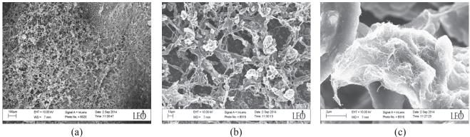
Fig. 3. SEM images of surface of MWCNT/chitosan based aerogels.
