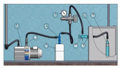
Fig. 1. The scheme of installation for freeze-drying of samples: 1 – the vacuum pump VRD-4; 2 – ball valve; 3 – a vessel filled with liquid nitrogen; 4 – Glass trap placed in liquid nitrogen to condense water vapor coming from sublimation of ice; 5 – Vacuum gauge; 6 – freezer Exquisit; 7 – the vacuum valve; 8 – a rubber stopper; 9 – flask with frozen hydrogel.
