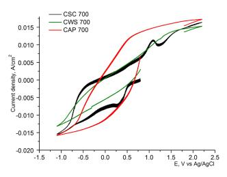
Fig. 4. CVA-curves of the test electrodes obtained by thermal carbonization.
