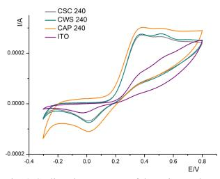
Fig. 6. Cyclic voltammograms of dopamine on the test electrodes obtained by hydrothermal carbonization.
