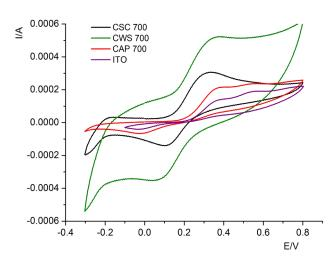
Fig. 5. Cyclic voltammograms of dopamine on the test electrodes obtained by thermal carbonization.
