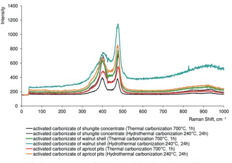
Fig. 2. Raman spectra of carbon containing electrode materials.
