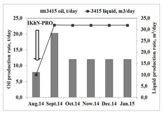
Fig. 5. Oil and liquid production rates for well 3415 after treatment of the bottomhole zone with the oil-displacing IKhN-PRO system.
