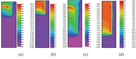
Fig. 7. Surface combustion: gas temperature  $T_g$  (0.02, x, r) (a) and nickel zinc ferrite concentration Fer1 (0.02, x, r) (b) at t = 0.02; and gas temperature  $T_g$  (0.04, x, r) (c) and nickel zinc ferrite concentration Fer1 (0.04, x, r) (d) at time t = 0.04. The calculations are presented when  $A_T = A_{O2} = A_{CO2} = 10$  and porosity is 0.05%. Slip intensity effect is  $A_u = 100$ .
