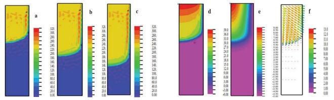
Fig. 5. Nickel zinc ferrite Fer(t, x, r) distributions at (a) -t = 0.2; (b) -t = 0.3, (c) -t = 0.4. The temperature of gas (d)  $-T_g(0.2, x, r)$ ; solid (e)  $-T_s(0.2, x, r)$  and velocity of gas (f) -u(0.2, x, r) distributions at t = 0.2 with porosity of 40%.
