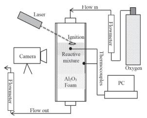
Fig. 1. Schematics of the experimental setup.
