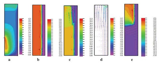
Fig. 8. Surface combustion: (a) – gas temperature  $T_g (0.1, x, r)$ ; (b) – nickel zinc ferrite concentration Fer1 (0.1, x, r) at t = 0.1; (c) – the carbon concentration C (0.02, x, r); (d) – gas velocity (0.02, x, r); (e) – nickel zinc ferrite concentration Fer1 (0.02, x, r) at t = 0.02. Fpr all these cases the parameters  $A_T = A_{O2} = A_{CO2} = 0$ , porosity of 0.05% and slip intensity effect is  $A_u = 0$ .
