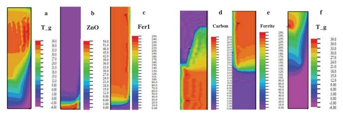
Fig. 6. (a) – Gas temperature  $T_g$  (0.2, x, r); (b) – zinc oxide ZnO (0.2, x, r); (c) – nickel zinc ferrite concentration Fer1 (0.2, x, r) at t = 0.2. (d) – Carbon C (0.1, x, r); (e) – nickel zinc ferrite Fer (0.1, x, r); (f) – concentration and gas temperature distribution  $T_g$  (0.1, x, r) at time t = 0.1 is presented when  $A_T = A_{02} = A_{C02} = 10$  and porosity is 40%. Slip intensity effect is  $A_u = 100$ .
