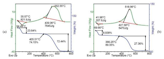
Fig. 2. a) DTA-TG curves for the carbon combustion at 20 °C/min heating rate, b) DTA-TG curves for the mixture with  $\alpha = 10$  at 20 °C/min heating rate.
