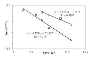
Fig. 3. Arrhenius plots for the carbon combustion (triangles) and combustion of  $\alpha = 10$  mixture (squares) at heating rates 5–25 °C/min.
