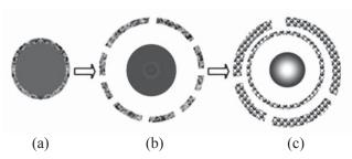
Fig. 4. Schematic of the melt-dispersion mechanism of combustion of nano aluminum particles at a high heating rate (>10<sup>6</sup> K/s) [11]: (a) aluminum core covered by the initial alumina shell; (b) fast melting of aluminum leads to spallation of the alumina shell; (c) unloading wave propagates to the center of the molten core of the Al particle and generates tensile pressure, which disperses small Al clusters.
