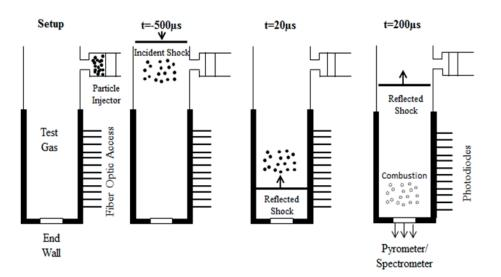
Fig. 1. Schematic of shock tube tests [6].
