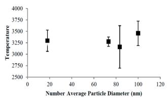
Fig. 2. Maximal particle temperature vs. size at  $1500 \pm 50$  K (20 atm, 20% O<sub>2</sub>:80% N<sub>2</sub>) [6].
