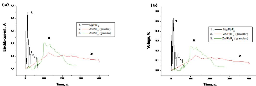
Fig. 8. The comparison of values of electric current and voltage in different systems of PRPS.
