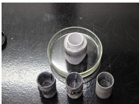
Fig. 4. External view of cathode-anode cells before and after experiments.
