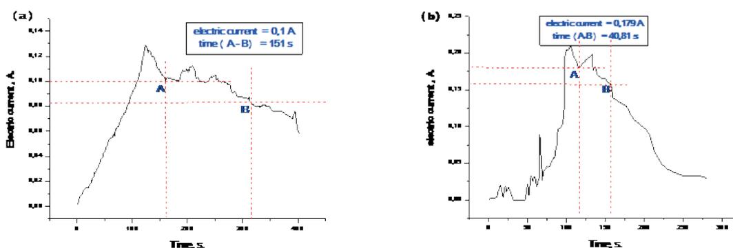
Fig. 7. The time dependence of electric current values for powder (a) and granular (b) zinc.
