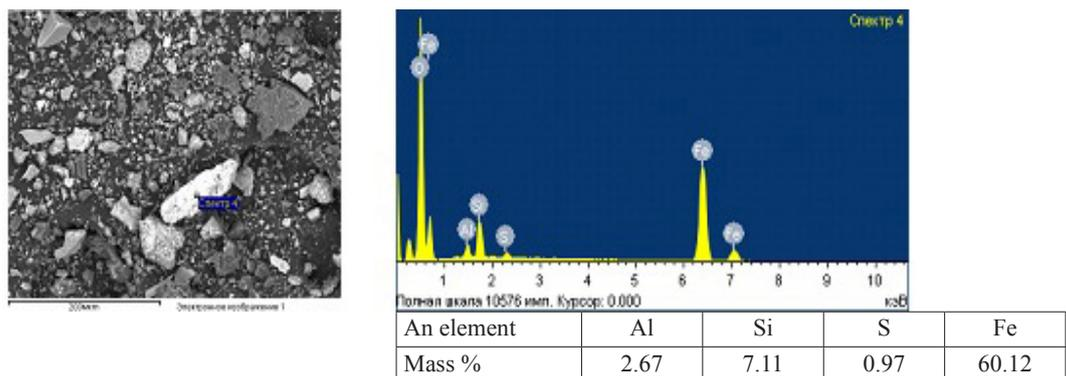
Fig. 9. An elemental composition of the internal overburden rock a) spectrum 1; b) spectrum 2; c) spectrum 3; d) spectrum 4.
