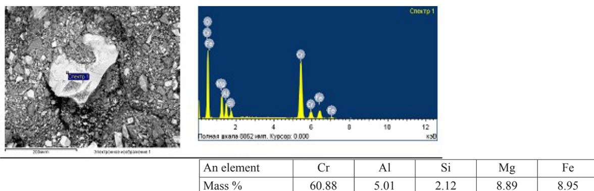
Fig. 10. The elemental composition of the calcined chromite pellets containing 10 % of the internal overburden rock and 2% of coal fines (spectrum 1).
