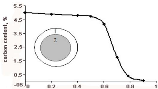
Fig. 5. Dependence of the carbon distribution in volume of the chromite pellets: 1 – a superficial light free-carbon layer; 2 – an internal dark carbon-containing layer.
