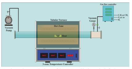
Fig. 1. The general scheme of the setup used in the method of TCVD.
