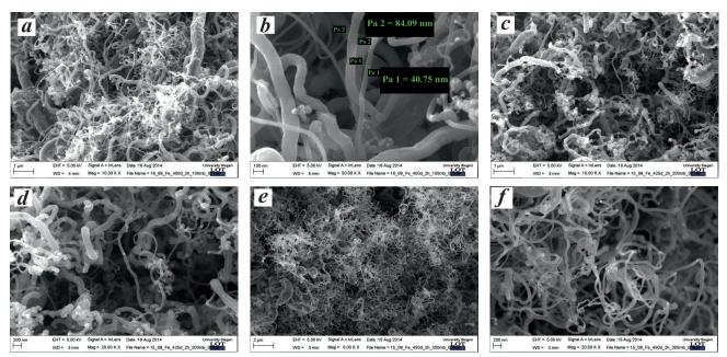
Fig. 5. SEM images of CNs on iron NP: a, b – 400 °C, 100 mbar; c, d – 425 °C, 200 mbar; e, f – 450 °C, 300 mbar.
