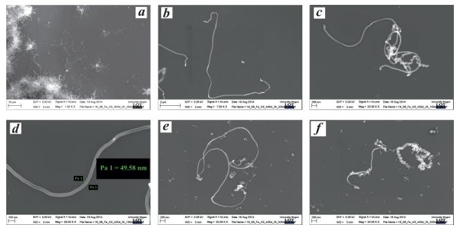
Fig. 6. SEM images of CNs on the separated iron NP: a, b – 400 °C, 100 mbar; c, d – 425 °C, 200 mbar; e, f – 450 °C, 300 mbar.
