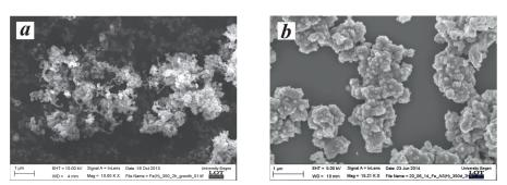
Fig. 4. SEM images of CNs on iron NP (a) and carbonated agglomerates of nanoclusters (b). Synthesis conditions: temperature – 350 °C, pressure – 500 mbar.
