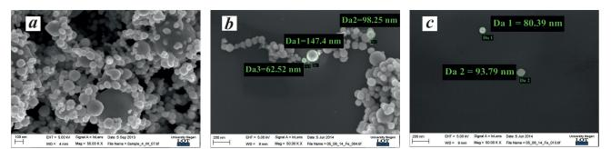
Fig. 2. SEM images of iron NP (a), agglomerates of nanoclusters (b) and individual nanoclusters (c) after separation in hexane.
