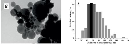
Fig. 3. TEM images of iron NPs (a) and histogram of size distribution of iron NPs (b).
