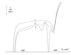
Fig. 9. Anodic VA curves for Ni $\rightarrow$ Cu deposits obtained at concentrations:  $c(Ni^{2+})$ ,  $10^{-4}$  M: 1 - 3;  $c(Cu^{2+})$ ,  $10^{-5}$  M: 1 - 0; 2 - 2; 3 - 4.
