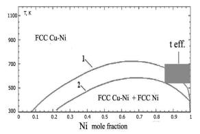
Fig. 10. Variants (1, 2) of low temperature fields of Cu–Ni phase diagram and effective temperature area for nano-sized bimetal.
