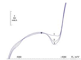
Fig. 4. Anodic VA curves for Co–Ni deposits obtained at simultaneous deposition time: 1) 15 s, 2) 30 s, 3) 45 s; at concentrations:  $c(\text{Co}^{2+}) = 9 \cdot 10^{-5} \text{ M}$ ,  $c(\text{Ni}^{2+}) = 2 \cdot 10^{-5} \text{ M}$ .
