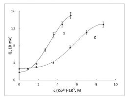
Fig. 7. Dependence of the quantity of electricity under anodic peak on  $Co^{2+}$  concentration for Ni $\rightarrow$ Co deposits, obtained from solution containing  $c(Ni^{2+})$ ,  $10^{-5}$  M: 1-9.; 2–13.
