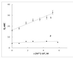
Fig. 6. Dependence of the quantity of electricity under anodic peak on Ni<sup>2+</sup> concentration for Co $\rightarrow$ Ni deposits obtained from solutions containing  $c(Co^{2+})$ , 10<sup>-5</sup> M: 1–13; 2–5.
