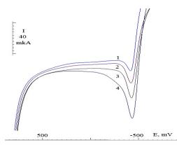
Fig. 3. Anodic VA curves for Ni $\rightarrow$ Co deposits obtained at concentrations: c (Ni<sup>2+</sup>) = 0.9 $\cdot$ 10<sup>-4</sup> M, c (Co<sup>2+</sup>), 10<sup>-5</sup> M: 1 - 0; 2 - 1; 3 - 2; 4 - 4.
