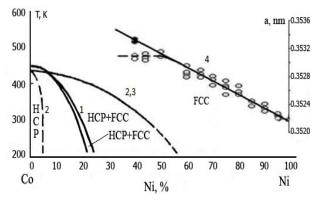
Fig. 5. Phase digram of the binary system Co-Ni (low temperature area) -1, 2 and fragment of PD of nanosized system (3) with dependence of lattice parameter on composition (4) [15].
