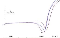
Fig. 2. Anodic VA curves for Co $\rightarrow$ Ni deposits obtained at concentrations:  $c(\text{Co}^{2+}) = 5 \cdot 10^{-5} \text{ M}(1), c(\text{Ni}^{2+}), 10^{-5} \text{ M}: 1-0; 2-1; 3-2.$
