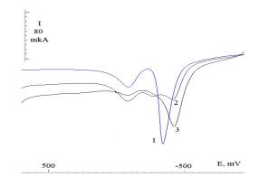
Fig. 8. Anodic VA curves for Cu $\rightarrow$ Ni deposits obtained at concentrations:  $c(\text{Cu}^{2+})$ ,  $10^{-4}$  M: 1 - 1,1; c (Ni<sup>2+</sup>),  $10^{-4}$  M: 1 - 0; 2 - 2; 3 - 6.
