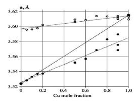
Fig. 11. Dependence of Ni  $(\bullet)$  and Cu  $(\circ)$  phases lattice parameters on the system composition.
