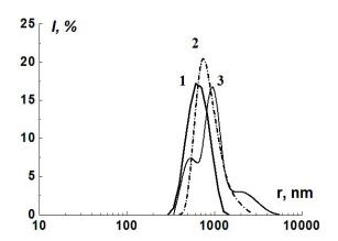
Fig. 1. Particles size distribution (r, nanometer) of the light scattering relative intensity indicator (I, %) in  $CaCl_2$  solutions (mol/l): 1 - 0.032; 2 - 0.48; 3 - 0.965.
