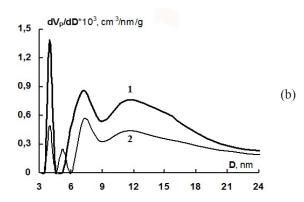
Fig. 5. Differential size curve distributions by the specific surface area ( $dS_{SA}/dD$ ,  $cm^2/nanometer/g$ ) (a) and the pore volume ( $dV_P/dD$ ,  $cm^3/nanometer/g$ ) (b) in samples of cement stones 1 and 2.
