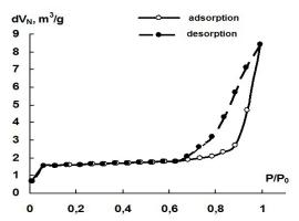
Fig. 3. Isotherms of low-temperature adsorption-desorption of nitrogen on a sample of a cement stone  $N_2$  1:  $dV_N$  – the volume of the sorbing and desorbing nitrogen,  $m^3/g$ ;  $P/P_0$  – change of nitrogen vapors pressure.
