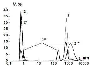
Fig. 2. Size distribution of the indicator of the particles relative volume (V, %) in initial (1)  $CaCl_2$  solution (0.032 mol/l), after mechanoactivation (2) and additional endurance within 1, 3 and 7 days (corresponding 2', 2"and 2"').
