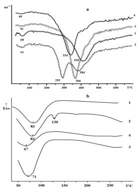
Fig. 1. The DTG (a) and DSC (b) curves of technical hydrolytic lignin obtained in inert atmosphere; T is the temperature: 1 – the KL sample; 2 – the EL sample; 3 – the NTL sample; 4 – the ML sample.
