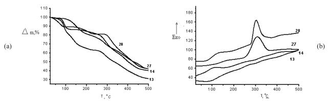
Fig. 4a. The TG curves of Samples 13, 14, 27 and 28. Fig. 4b. The DSC curves of Samples 13, 14, 27 and 28.
