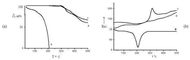
Fig. 3a. The TG curves of Samples 7–9. Fig. 3b. The DSC curves of Samples 7–9.
