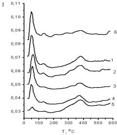
Fig. 6. The TVA curves of the THL samples impregnated with the DMSO/water binary mixture: 1 - DMSO + THL, sample weight is 0.0454 g; 2 - 70% of DMSO + 30% of water + THL; 3 - 50% of DMSO + 50% of water + THL; 4 - 30% of DMSO + 70% of water + THL; 5 - Water + THL; 6 - 70% of DMSO + 30% of water at 70 °C. The weight loss of the studied sample is 90–95% from the initial sample weight.
