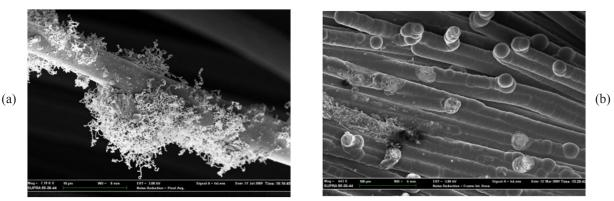
Fig. 4. Carbon fibers decorated with CNT. (a): SWCNT. (b): MWCNT.
