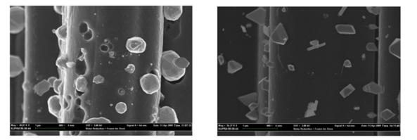
Fig. 2. Decoration of CNF by MS. (a): with Co nanoparticles. (b): with Ni nanoparticles.
