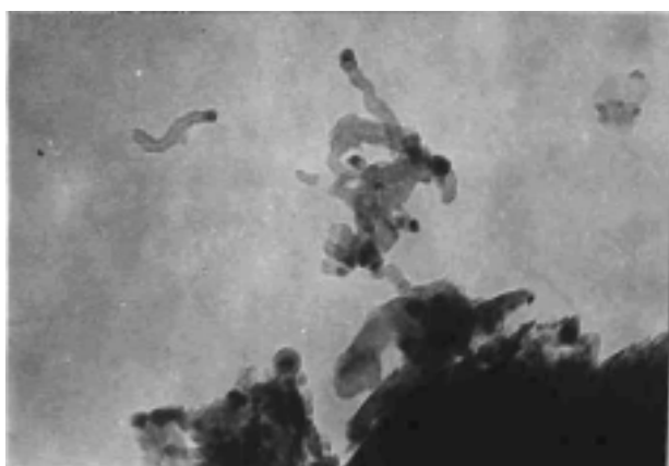
Fig. 4. 1% Ni/clay catalyst carbonized at 873 K, d = 120\text{-}140 \text{ \AA}
