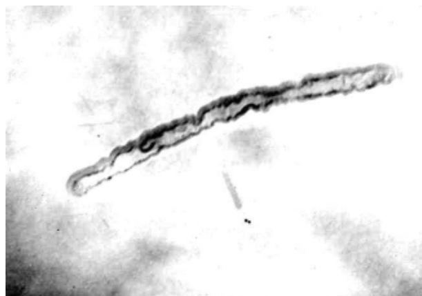
Fig. 6. After desorption of the \text{SO}_2 adsorbed at 423 K from 1% Ni/clay catalyst carbonized at 873 K
