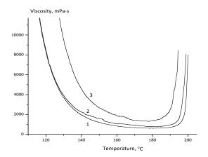
Fig. 4. Viscosity-temperature plots for PN-50 resin: untreated (1); heated for 3 h in vacuum (2); heated for 3 h in air (3).
