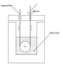
Fig. 1. Principal scheme of solvent free impregnation process.
