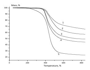
Fig. 5. TGA curves for cured PN-50 resin/DAEBA mixtures with various DAEBA content (mass.%): 0% (1); 10% (2); 33% (3); 50% (4); 100% (5).
