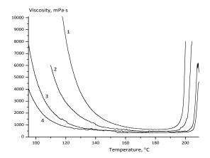
Fig. 3. Viscosity-temperature plots curves for PN-50 resin/DPEBA mixtures with various DPEBA content (mass.%): 0% (1); 20% (2); 33% (3); 50% (4).
