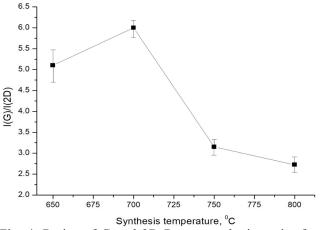
Fig. 4. Ratios of G and 2D Raman peaks intensity for different synthesis temperatures.
