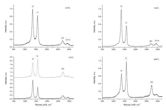
Fig.1. Raman spectra of MWCNTs synthesized on diatomite at different temperatures.
