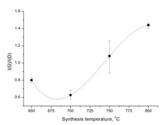
Fig. 3. The evolution of I(G)/I(D) ratio with the synthesis temperature.
