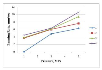
Fig. 4. Graph of the dependence of the burning rate on the pressure of the nitrogen gas: 1 – AN/MgAl; 2 – AN/MgAl/TiO<sub>2</sub>; 3 – AN/MgAl/ZrO<sub>2</sub>; 4 – AN/MgAl/Cr<sub>2</sub>O<sub>3</sub>.
