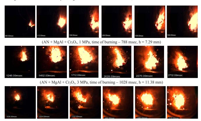
$(AN + MgAl + Cr_2O_3, 5 MPa, time of burning - 480 msec, h = 11.31 mm)$ Fig. 3. Cinegrams of combustion of gas generator based on  $AN/MgAl/Cr_2O_3$  at 1 MPa, 3 MPa and 5 MPa.
