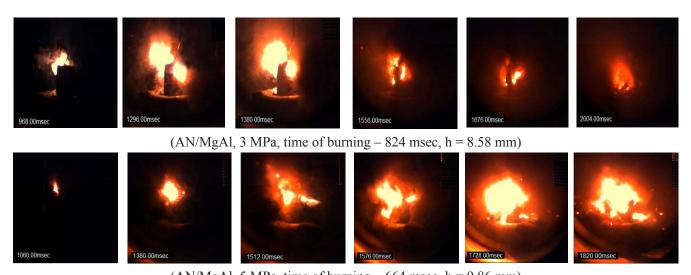
(AN/MgAl, 5 MPa, time of burning -664 msec, h = 9.86 mm) Fig. 2. Burning cinegram of the AN/MgAl - based gas generators at a pressure of 3 MPa and 5 MPa.
