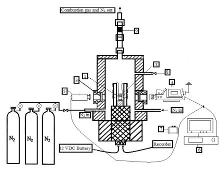
Fig. 1. Scheme of the combustion chamber under pressure: 1 – sample; 2 – nichrome wire; 3 – window; 4 – high-speed video camera; 5 – camera; 6 – transformer; 7 – PC; 8 – system for pressure control; 9 – filter.
