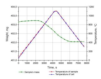
Fig. 7. Changes of sample's mass during heating.
