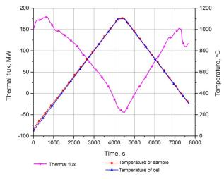
Fig. 8. Changes of heat flux of sample during heating.
