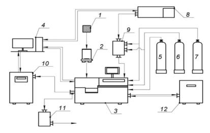
Fig. 2. Schematic diagram of the experimental complex: 1 – sample; 2 – analytical scales; 3 – thermal gravimetrical analyzer; 4 – computer; 5 – reaction gas; 6 – purge gas; 7 – shielding gas; 8 – humidity generator; 9 – mixing chamber; 10 – mass spectrometer; 11 – gas filter; 12 – cryostat.
