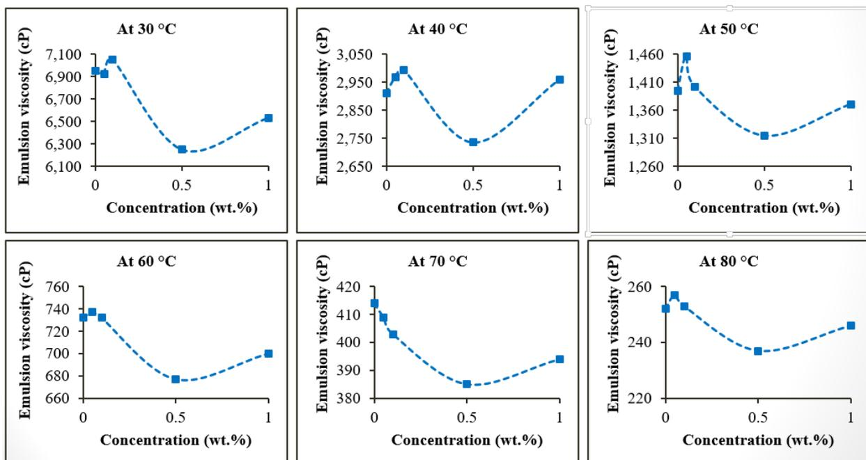
Fig. 4. Effect of nanofluid on emulsion viscosity.
