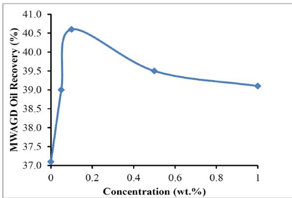
Fig. 3. Average oil recovery under MWAGD under microwave heating for  $\text{Al}_2\text{O}_3$  nanoparticles.
