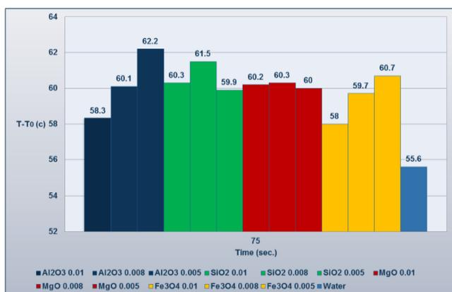
Fig. 1. Temperature alteration of deionized water and different water/nanofluid mixtures under microwave radiation
