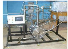
Fig. 5. Different types of pilot matrix converters with gas flows up to  $10 \text{ m}^3/\text{h}$ .
