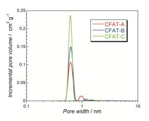
Fig. 4. Pore size distribution for polyHIPE derived carbons. Reprinted with permission for Ref. [17]. Copyright 2016, American Chemical Society.
