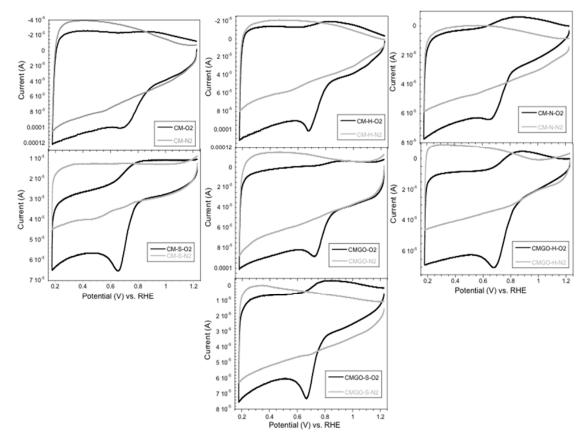
Fig. 9. Cyclic voltammograms measured using rotating ring-disk electrode in 0.10 M KOH at scan rate of 5 mV s<sup>-1</sup> for the materials studied. Reprinted with permission from Ref. [18]. Copyright 2017, American Chemical Society.
