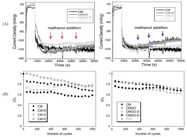
Fig. 11. A) Chronoamperometry response for methanol crossover at the potential of the maximum of the oxygen reduction humps; B) Stability of carbon foam (CM) and its modified counterparts and Pt/C in the ORR over 1000 cycles. Adapted with permission from Ref. [18]. Copyright 2017, American Chemical Society.
