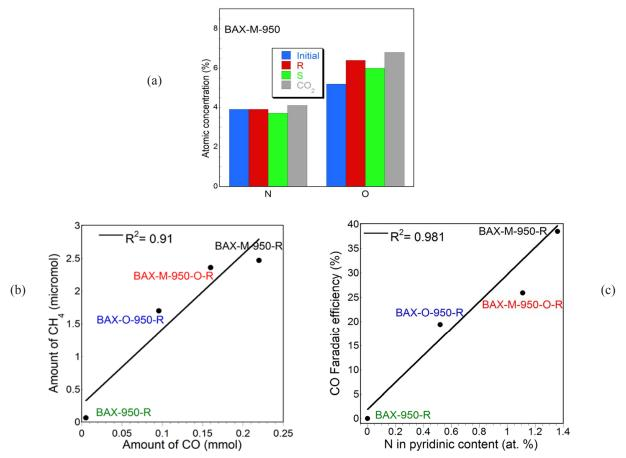
Fig. 3. A) Nitrogen and oxygen content on the surface of the initial sample, reduced in  $N_2$  saturated electrolyte – R; Stabilized in  $N_2$  saturated electrolyte – S and after  $CO_2$  electroreduction –  $CO_2$ ; B) Dependence of CO FE on the content of nitrogen in pyridinic groups; C) Dependence of the amount of  $CH_4$  formed on the amount of CO formed. Reprinted with permission from Ref. [14]. Copyright 2017, Elsevier.
