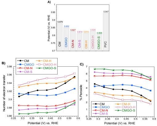
Fig. 10. Comparison of the onset potential (A), number of electron transfer (B) and the percentage of peroxide detected in the cells (C). Reprinted with permission from Ref. [18]. Copyright 2017, American Chemical Society.
