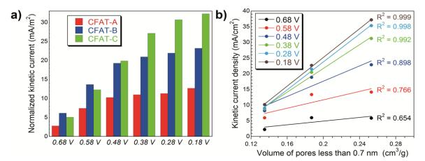
Fig. 7. a) Normalized kinetic current densities per  $S_{BET}$  surface area of the polyHIPEs carbons; b) Dependence of the kinetic current density vs. volume of pores smaller than 0.7 nm. Reprinted with permission for Ref. [17]. Copyright 2016, American Chemical Society.
