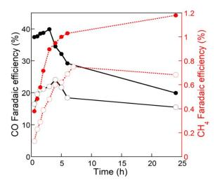
Fig. 2. The FE for CO and  $CH_4$  measured on BAX-M-950. Open symbol-initial sample; closed symbol – after 4 h of reduction at – 0.86 vs. RHE in N<sub>2</sub> saturated electrolyte).
