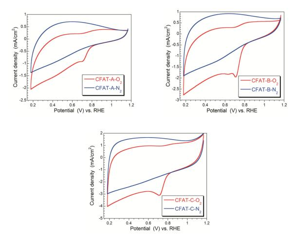
Fig. 5. Cyclic voltammograms on modified glassy carbon RDE in 0.10 M KOH at scan rate of 5 mV/s for the materials studied. Reprinted with permission for Ref. [17]. Copyright 2016, American Chemical Society.
