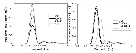
Fig. 8. Pore size distributions for carbon foam (CM) and its modified counterparts. Adapted with permission from Ref. [18]. Copyright 2017, American Chemical Society.
