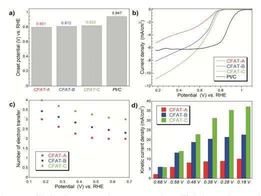
Fig. 6. a) Onset potentials; b) Linear sweep voltammograms on the modified glassy carbon RDE in O<sub>2</sub>-saturated 0.10 M KOH at 2000 rpm and scan rate of 5 mV/s; c) Number of electron transfer versus potential and d) Kinetic current density for the materials studied. Reprinted with permission for Ref. [17]. Copyright 2016, American Chemical Society.
