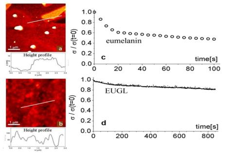
Fig. 5. Non-contact AFM images (5  $\mu$ m × 5  $\mu$ m) with corresponding height profile on a line of about 3  $\mu$ m on: (a) – EU; (b) – EUGL. Time dependent decay of the electrical conductivity on the EU – (c) and EUGL films – (d), at a fixed voltage (100 V for the EU, 100 mV for the EUGL). Adapted from [35].
