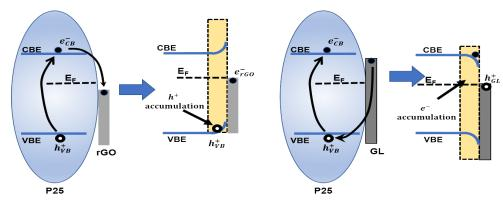
Fig. 6. Pictorial representation of the charge-transfers proposed for  $TiO_2/rGO$  (left) and  $TiO_2/GL$  (right) composites. CBE and VBE are conduction and valence band, respectively. Yellow regions represent the sub-surface accumulation regions for electrons in P25.
