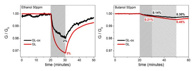
Fig. 4. Comparison between the response of the chemiresistive device based on  $GL_{ox}$  (black curve) and GL films (red curve) toward ethanol (right panel) and n-butanol (left panel). Adapted from [27].
