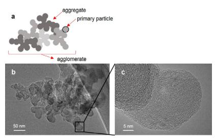
Fig. 1. Structure of CB (a), at micro (b) and nanoscale (c) level.
