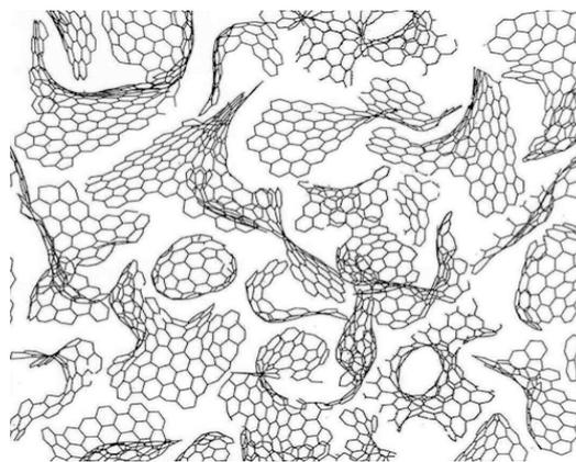
Fig. 4. Schematic illustration of a model for the structure of non-graphitizing carbons based on fullerene-like elements [7].
