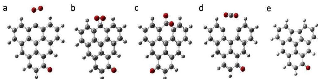
Fig. 6. Structures selected from computer simulation by Radovic et al. of the reaction between O<sub>2</sub> and the zig-zag edge of a char, to produce CO<sub>2</sub> [44].
