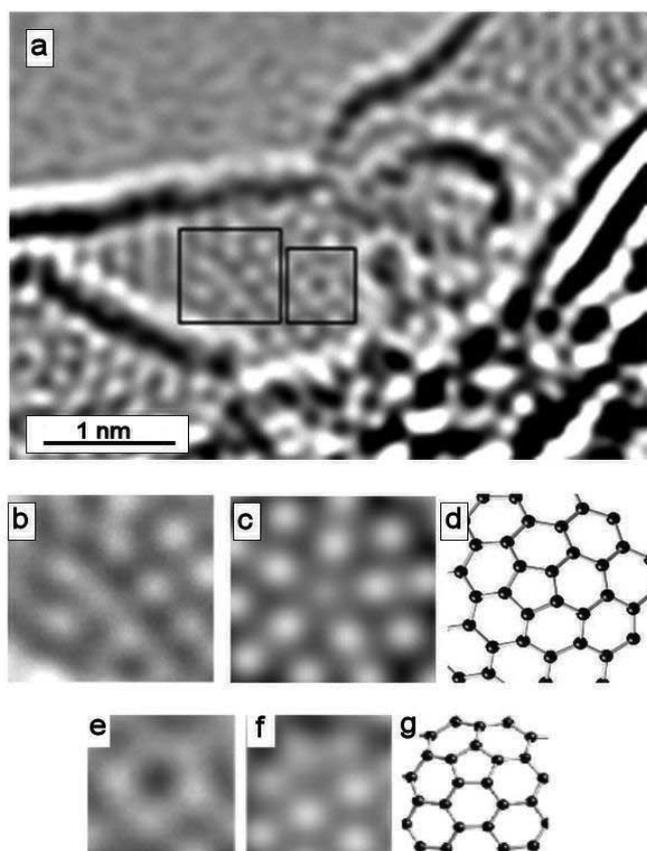
Fig. 5. (a) Aberration-corrected micrograph of activated carbon heated to 2000 °C; (b) Enlarged region showing pentagonal arrangement of spots; (c) Simulated image of structure shown in (d); (e) Second region showing pentagonal arrangement; (f) Simulated image of structure shown in (g) [24].
