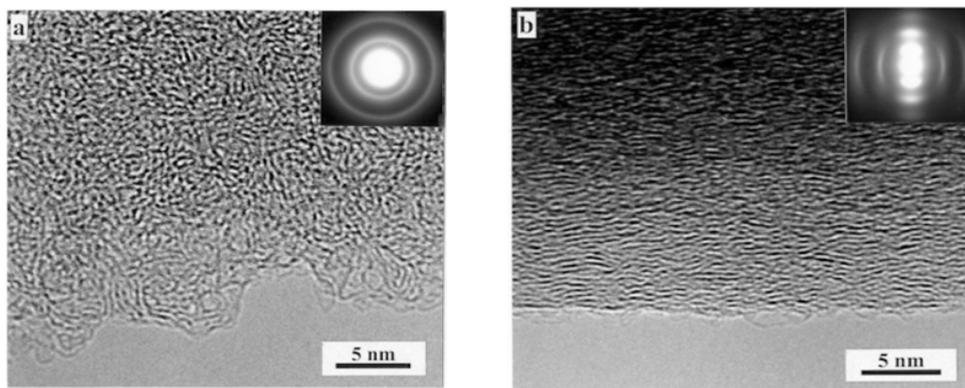
Fig. 2. (a) High resolution TEM image of carbon prepared by pyrolysis of sucrose in  $N_2$  at 1000 °C; (b) carbon prepared by pyrolysis of anthracene at 1000 °C. Insets show selected area diffraction patterns [5].
