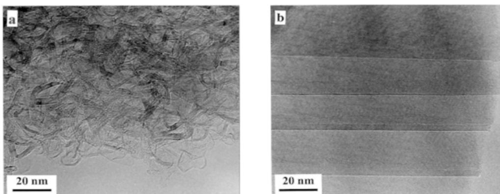
Fig. 3. Micrographs of (a) sucrose carbon and (b) anthracene carbon following heat treatment at 2300 °C [6].
