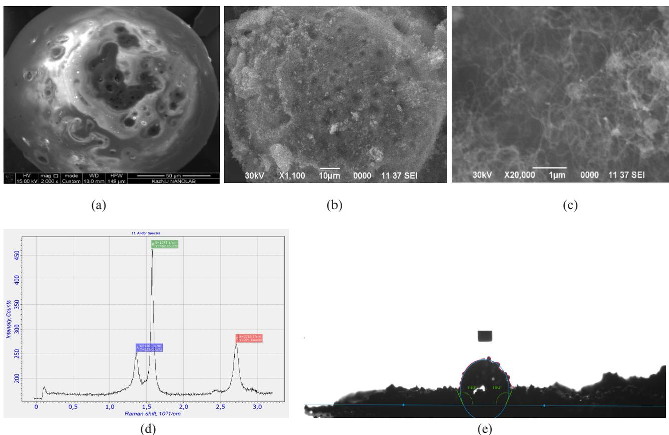
Fig. 2. (a) – SEM image of the surface of cenosphere before the synthesis of CNTs; (b) – SEM image of the surface of cenosphere after synthesis of CNTs; (c) – CNTs synthesized on a  $\text{Fe@P}'_{100/500}$  catalyst from HDPE at polyethylene decomposition temperature of 450 °C; (d) – Raman spectrum of CNTs; (e) – snapshot of a drop of water on the surface of cenospheres coated with carbon nanotubes.
