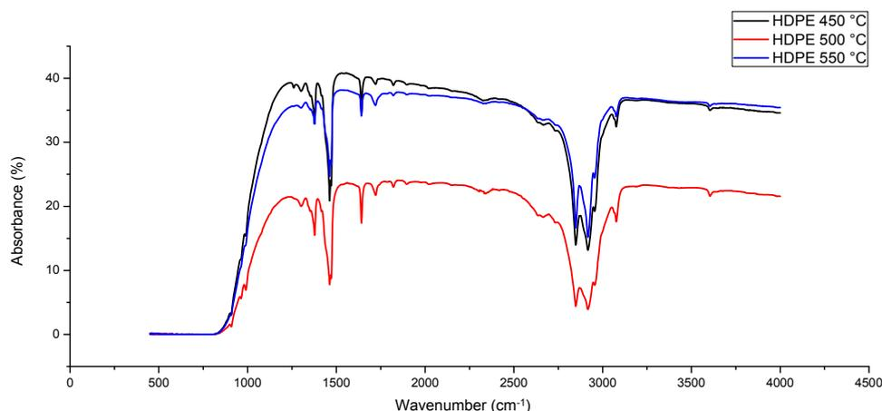
Fig. 1. IR-spectra of the decomposition products of HDPE at various temperatures: black – 450 °C; red – 500 °C; blue – 550 °C.
