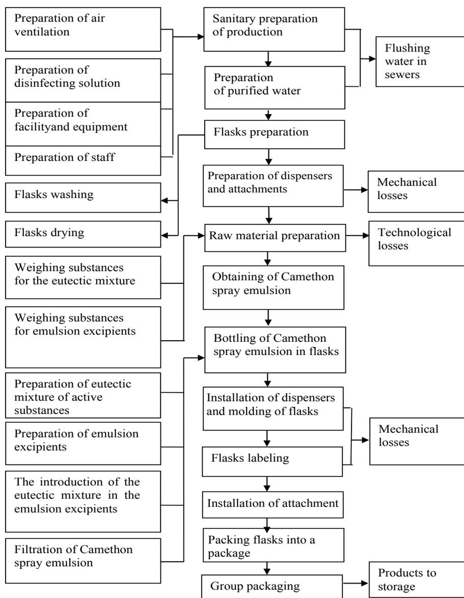
Scheme. Technological process scheme for the production of the drug “Camethon-Spray”.
