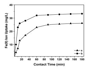
Fig. 5. Effect of adsorption time on Ni/Cr (a) and Ni/Cr-  $[\alpha\mathchar`-SiW_{12}O_{40}]$  (b) LDHs.
