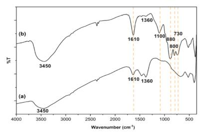
Fig. 2. FTIR spectra of Ni/Cr (a) and Ni/Cr- $[\alpha$ -SiW<sub>12</sub>O<sub>40</sub>] (b) LDHs.
