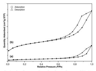
Fig. 3. The nitrogen adsorption desorption on Ni/Cr (a) and Ni/Cr-[ $\alpha$ -SiW<sub>12</sub>O<sub>40</sub>] (b).
