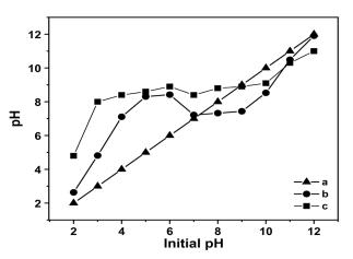
Fig. 4. pHpzc graph: initial pH (a), Ni/Cr (b) and Ni/Cr- $[\alpha$ -SiW<sub>12</sub>O<sub>40</sub>] (c).
