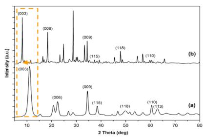
Fig. 1. XRD powder patterns of Ni/Cr (a) and Ni/Cr- $[\alpha$ -SiW<sub>12</sub>O<sub>40</sub>] (b) LDHs.
