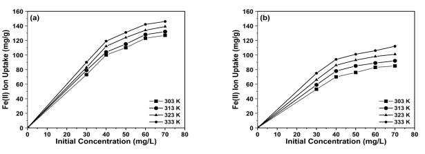
Fig. 6. Effect of iron(II) concentration and temperature adsorption on Ni/Cr (a) and Ni/Cr-[α-SiW<sub>12</sub>O<sub>40</sub>] (b) LDHs.
