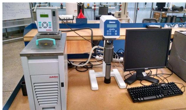
Fig. 3. Rheometer and Heat Bath Setup.
