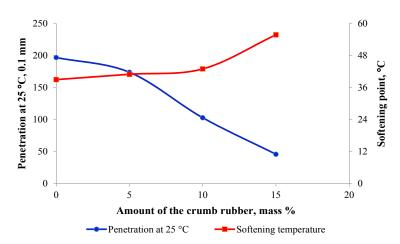
Fig. 4. Dependences of penetration at 25 °C (a) and softening point (b) of vacuum residue oxidation products for 3 h on the amount of the crumb rubber.
