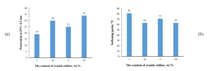
Fig. 5. Penetration at 25 °C (a) and softening point (b) of vacuum residue oxidation products for 3 h at various contents of crumb rubber.
