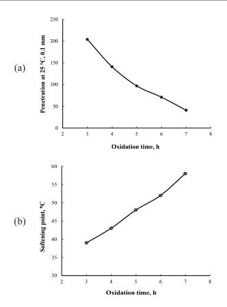
Fig. 2. Dependences of penetration at 25 °C (a) and softening point (b) of vacuum residue oxidation products with the addition of 15 wt.% crumb rubber (0.6-1.0 mm) from the duration of oxidation.
