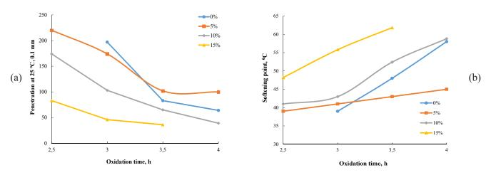
Fig. 3. Dependences of penetration at 25 °C (a) and softening point (b) of vacuum residue oxidation products on the processing time with the addition of various amounts of crumb rubber.
