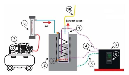
Fig. 1. Scheme of the installation for the oxidation of vacuum residue: 1 - a cylindrical steel reactor; 2 - an electric tube furnace; 3 - a temperature controller with a temperature controller; 4 - thermocouples; 5 - power supply; 6 - temperature controller; 7 - compressor; 8 - airflow meter; 9 - branch pipe for air supply; 10 - the flow of exhaust gaseous products.
