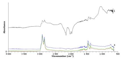
Fig. 7. IR spectra of crumb rubber (1), vacuum residue (2) and its oxidation products without (3) and with the addition of crumb rubber (4).
