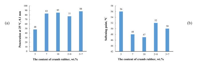
Fig. 6. Penetration at 25 °C (a) and softening point (b) of vacuum residue oxidation products for 2 h at various contents of crumb rubber.
