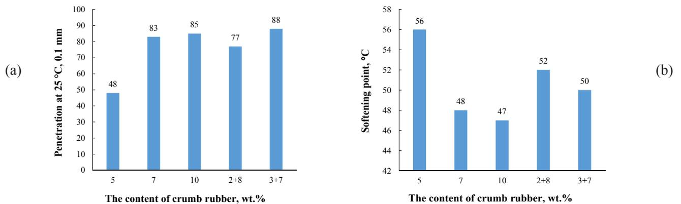
Fig. 6. Penetration at 25 °C (a) and softening point (b) of vacuum residue oxidation products for 2 h at various contents of crumb rubber.
