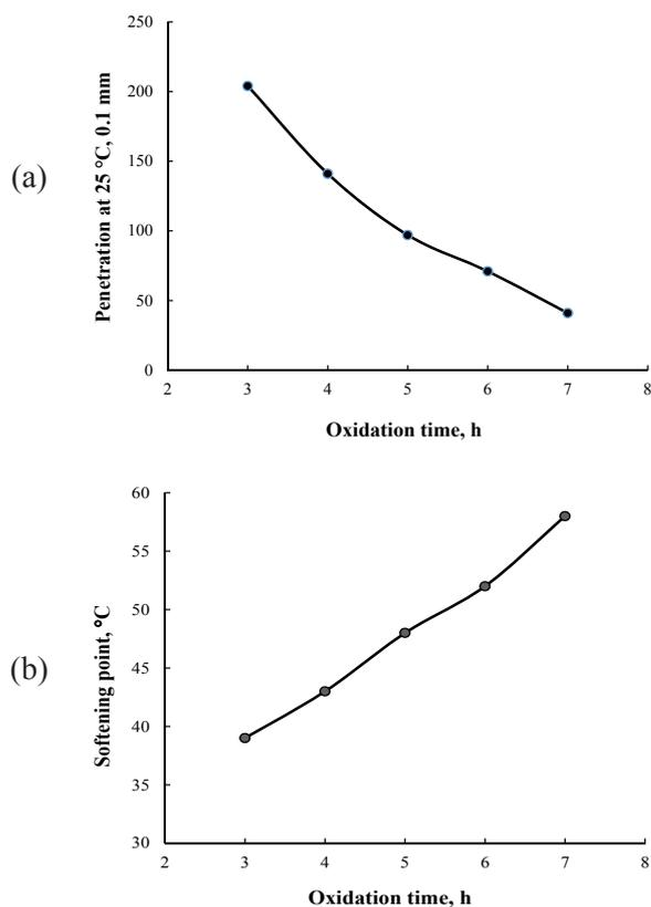
Fig. 2. Dependences of penetration at 25 °C (a) and softening point (b) of vacuum residue oxidation products with the addition of 15 wt.% crumb rubber (0.6–1.0 mm) from the duration of oxidation.
