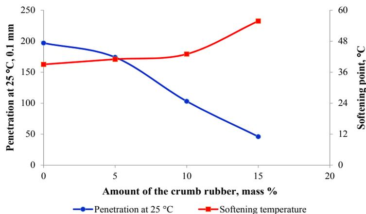
Fig. 4. Dependences of penetration at 25 °C (a) and softening point (b) of vacuum residue oxidation products for 3 h on the amount of the crumb rubber.
