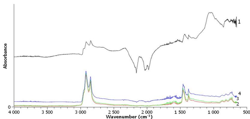
Fig. 7. IR spectra of crumb rubber (1), vacuum residue (2) and its oxidation products without (3) and with the addition of crumb rubber (4).
