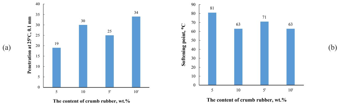
Fig. 5. Penetration at 25 °C (a) and softening point (b) of vacuum residue oxidation products for 3 h at various contents of crumb rubber.
