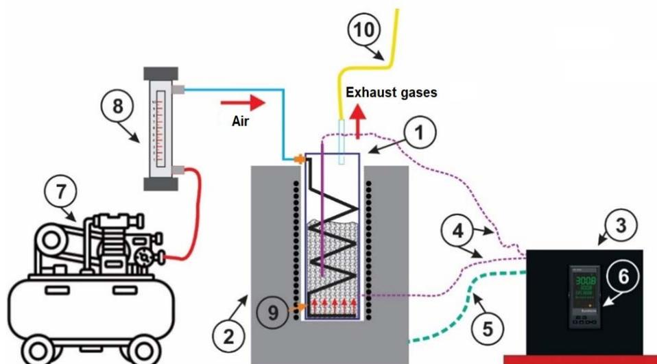
Fig. 1. Scheme of the installation for the oxidation of vacuum residue: 1 – a cylindrical steel reactor; 2 – an electric tube furnace; 3 – a temperature controller with a temperature controller; 4 – thermocouples; 5 – power supply; 6 – temperature controller; 7 – compressor; 8 – airflow meter; 9 – branch pipe for air supply; 10 – the flow of exhaust gaseous products.
