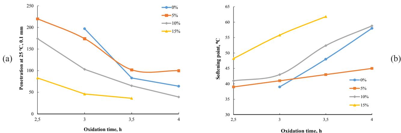
Fig. 3. Dependences of penetration at 25 °C (a) and softening point (b) of vacuum residue oxidation products on the processing time with the addition of various amounts of crumb rubber.
