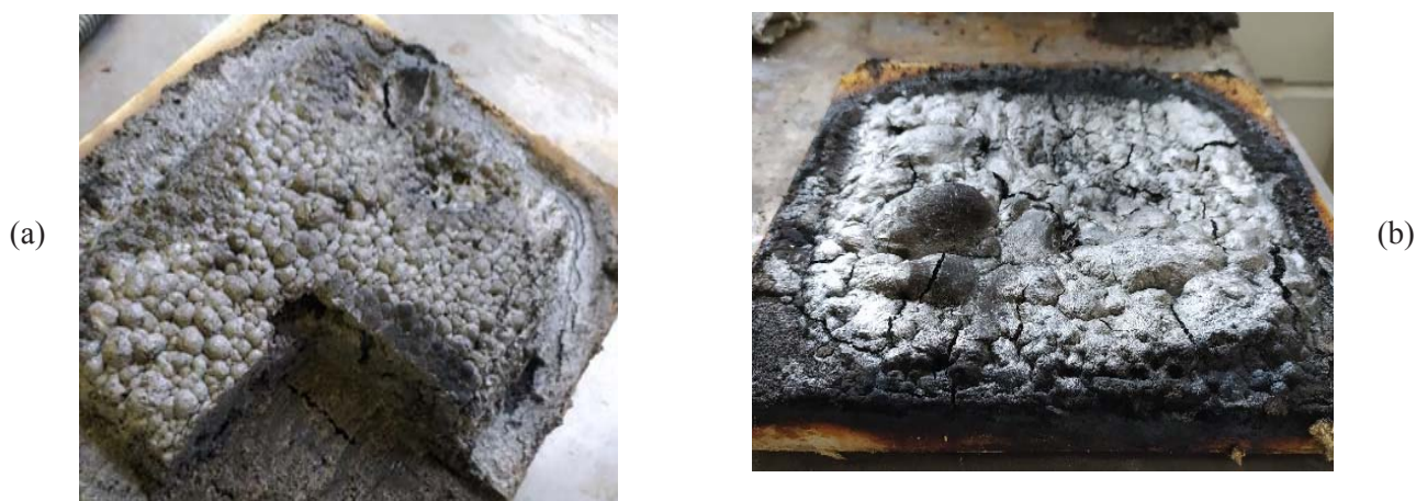
Fig. 3. The appearance of the foamed thermal insulation layer on the surface of wood after fire tests: (a) – 2; (b) – 4 (sample numbers listed in Table).
