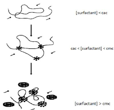
Fig. 2. Conformation of HPMC and surfactant complexes [Ref. 106].
