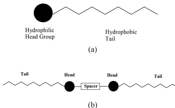
Fig. 1. Schematic illustration of the (a) conventional and (b) gemini surfactants.
