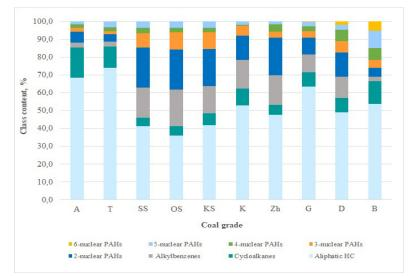
Fig. 5. Distribution of organic compounds in coal samples of different ranks for grain size class (-0.04) mm, recorded by means of GC/GC-FID.
