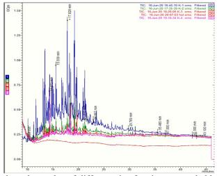
Fig. 2. Chromatograms of K rank coal samples of different size fractions, recorded by means of GC-MS: 1 - (-0.04) mm; 2 - (-0.063+0.04) mm; 3 - (-0.1+0.063) mm; 4 - (-0.2+0.1) mm.
