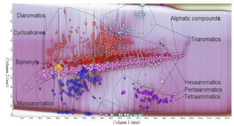
Fig. 4. Chromatogram of the sample of Zh rank coal of the grain size class (-0.04) mm recorded by means of GC/GC-FID.
