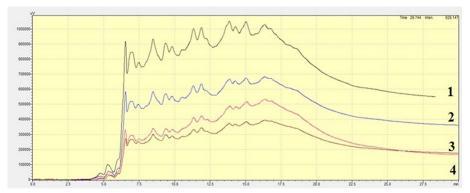
Fig. 1. Chromatograms of the coal samples of K rank with different particle size fractions, recorded by means of HPLC: 1 - (-0.04) mm; 2 - (-0.063+0.04) mm; 3 - (-0.1+0.063) mm; 4 - (-0.2+0.1) mm.
