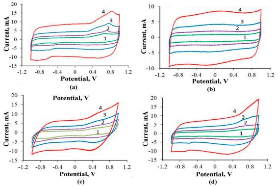
Fig. 2. CVA curves for asymmetric cells with the electrodes made of the corresponding matrix and NC  $Co_{0.5}Ni_{0.5}(OH)_2/MWCNT$  (5 wt.% MH) (a) and  $Co_{0.5}Ni_{0.5}(OH)_2/MWCNT$ -f (5 wt.% MH) (b);  $Co_{0.5}Ni_{0.5}(OH)_2/MWCNT$  (10 wt.% MH) (c) and  $Co_{0.5}Ni_{0.5}/MWCNT$ -f (10 wt.% MH) (d), at the potential scanning rates: 1 - 10 mV/s; 2 - 20 mV/s; 3 - 40 mV/c; 4 - 80 mV/s.
