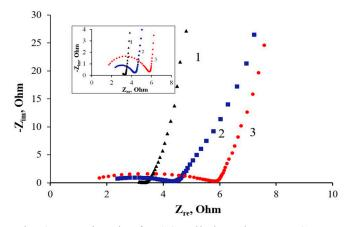
Fig. 3. Nyquist plot for SC cells based on MWCNTs and NC on this basis: 1 - symmetrical cell with electrodes based on MWCNT; 2-3 - asymmetric cells with working electrodes based on NC with the composition  $Co_{0.5}Ni_{0.5}(OH)_2/MWCNT$  (5 and 10 wt.% MH, respectively) and counter electrodes based on MWCNTs.
