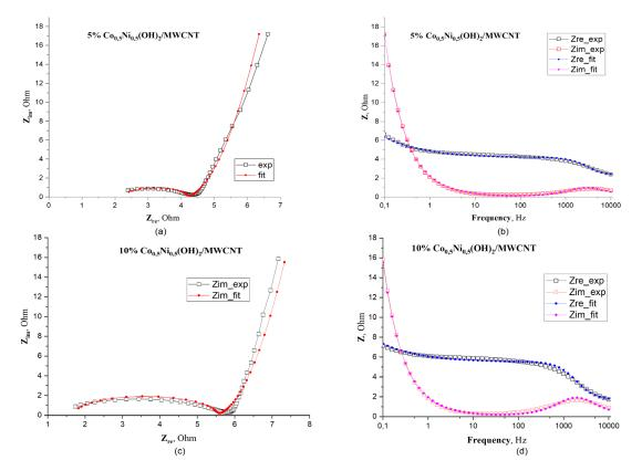
Fig. 5. Comparison of the experimental Nyquist (a, c) and Bode (b, d) dependences with the results of modeling for electrochemical cells with the working electrodes based on NC with different MH-filler content: 5 wt.% (a, b); 10 wt.%. (c, d).
