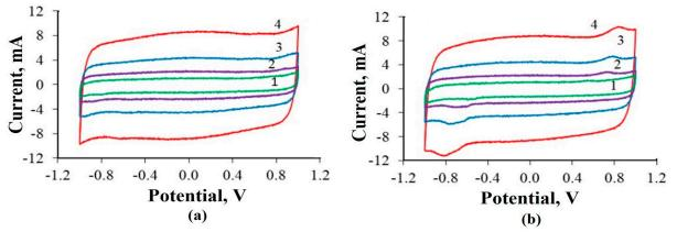
Fig. 1. CVA curves for symmetrical cells with the electrodes made of MWCNT (a) and MWCNT-f (b), at scanning rates: 1 - 10 mV/s; 2 - 20 mV/s; 3 - 40 mV/s; 4 - 80 mV/s.
