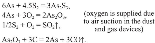
In general, sulphide and oxide compounds of other non-ferrous metals, in particular, copper, lead and zinc, which are contained in initial ledge gold ore and flux, may also participate in the above mentioned physical and chemical processes during the RPS Process refractory gold ore smelting.
