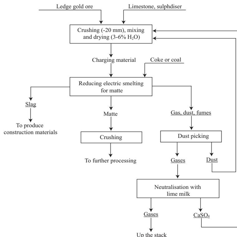
Fig. 1. Refractory Ledge Gold Ore Processing RPS Process Flow Sheet.
