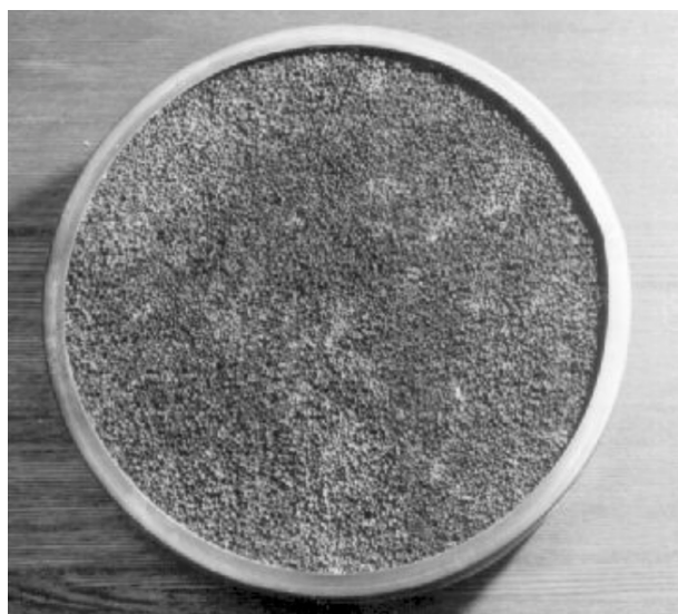
Fig. 6. Catalytic block in the metal drum.
