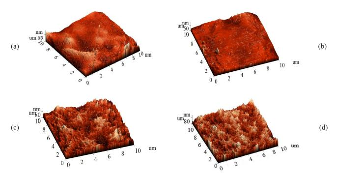
Fig. 5. AFM images of gelatin-coated alginate sample: alginate (a); alginate-gelatin (b); alginate-gelatin pH=6.86 (c); alginate-gelatin pH=9.18 (d).
