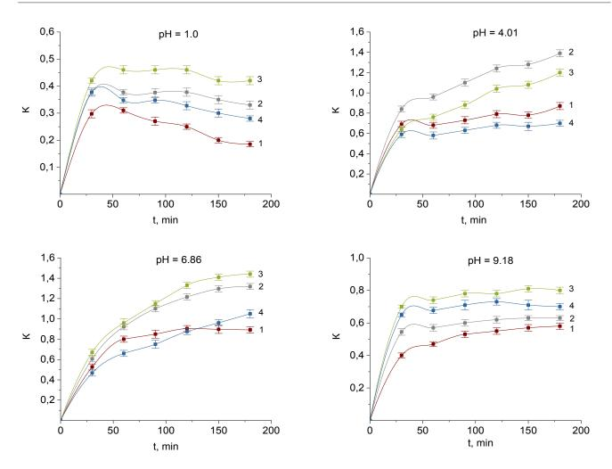
Fig. 1. Swelling of alginate particles under simulated gastrointestinal conditions:  $1 - CaCl_2$  (0.5 %);  $2 - CaCl_2$  (1%);  $3 - CaCl_2$  (1.5%);  $4 - CaCl_2$  (2%).
