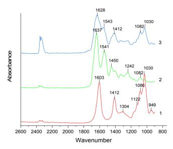
Fig. 4. FTIR spectrum of sodium alginate (1), gelatin (2), gelatin-coated alginate particle (3).
