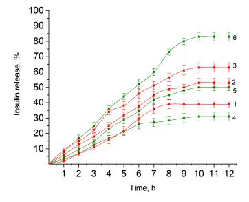
Fig. 3. Insulin release from alginate and gelatin-coated alginate particles under simulated gastrointestinal conditions: 1 - pH=4.01; 2 - pH=6.86; 3 - pH=9.18 for alginate particles; 4 - pH=4.01; 5 - pH=6.86; 6 - pH=9.18 for gelatin-coated alginate particles.
