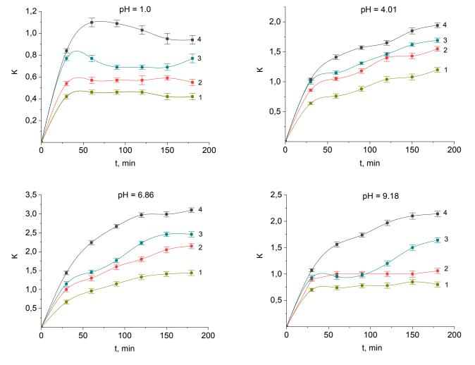
Fig. 2. Swelling of gelatin-coated alginate particles under simulated gastrointestinal conditions: 1 – alginate (1%); 2 – alginate-gelatin (2%); 3 – alginate-gelatin (5%); 4 – alginate-gelatin (8%).
