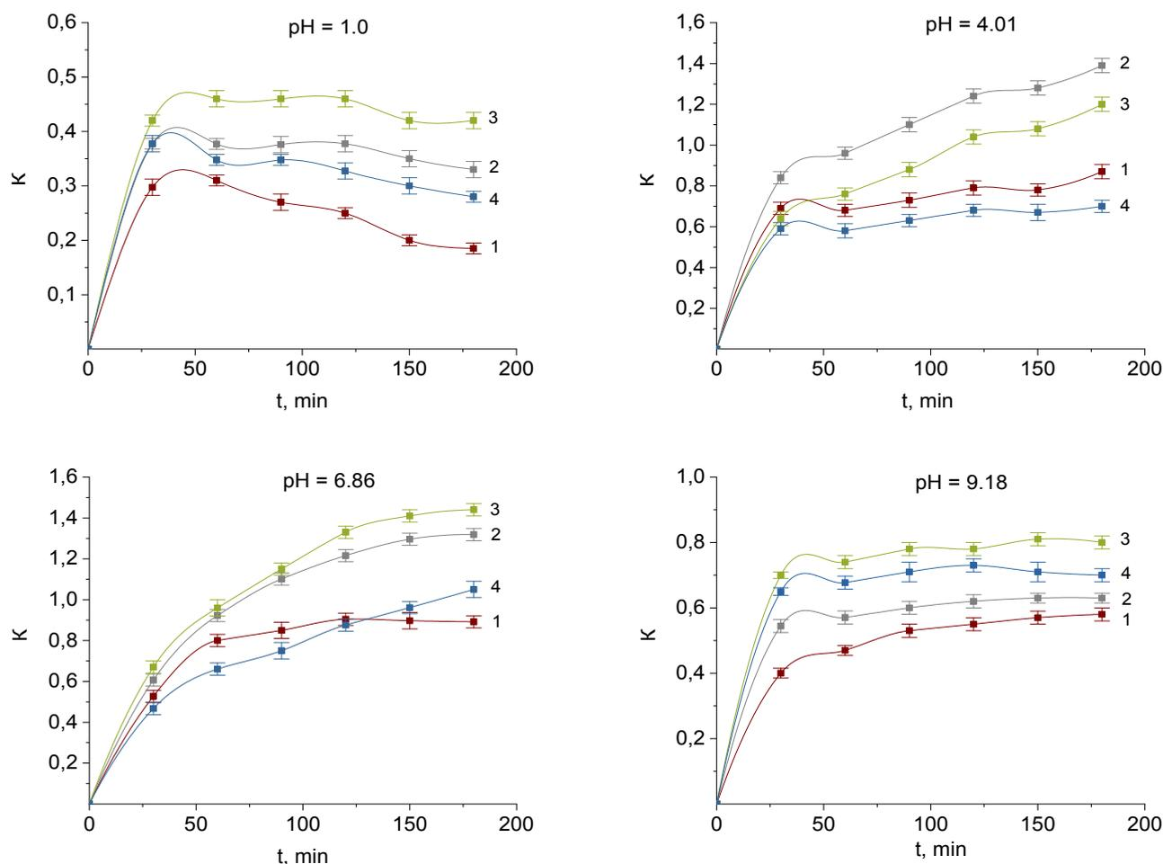
Fig. 1. Swelling of alginate particles under simulated gastrointestinal conditions: 1 – CaCl<sub>2</sub> (0.5 %); 2 – CaCl<sub>2</sub> (1%); 3 – CaCl<sub>2</sub> (1.5%); 4 – CaCl<sub>2</sub> (2%).
