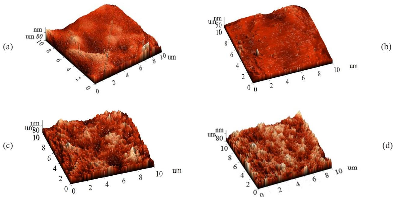
Fig. 5. AFM images of gelatin-coated alginate sample: alginate (a); alginate-gelatin (b); alginate-gelatin pH=6.86 (c); alginate-gelatin pH=9.18 (d).
