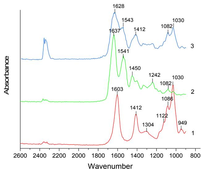
Fig. 4. FTIR spectrum of sodium alginate (1), gelatin (2), gelatin-coated alginate particle (3).
