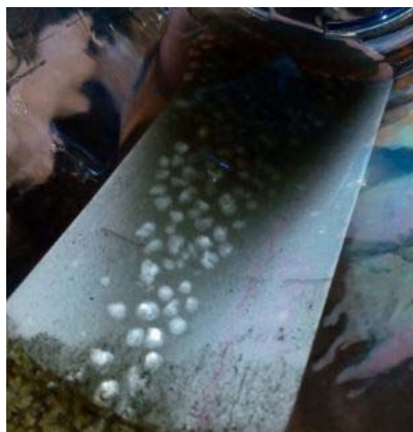
Fig. 2. Fish eyes (swollen polymer particles) in the sample taken from a mixing vessel in field conditions.
