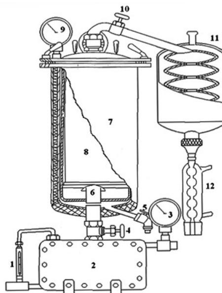
**Fig. 1.** Diagram of a barothermal installation: 1 – water level indicator; 2 – steam generator; 3 – steam generator pressure indicator; 4 – valve for allowing steam into the reactor; 5 – lower exhaust valve; 6 – steam distributor; 7 – reactor; 8 – container; 9 – reactor pressure indicator; 10 – upper exhaust valve; 11 – water refrigerator; 12 – reverse water refrigerator.
