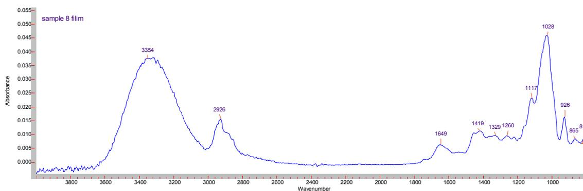
**Fig. 1.** IR spectrum of pullulan film.
