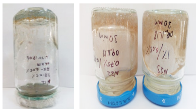
Fig. 7. Formed gels obtained by combined mixing of polymer (HPAM) and crosslinker during 30 min. Crosslinker concentration 0.05 wt.%. Polymer concentration varies from left to right: 1 – 0.5 wt.%; 2 – 0.75 wt.%; 3 – 1 wt.%.
