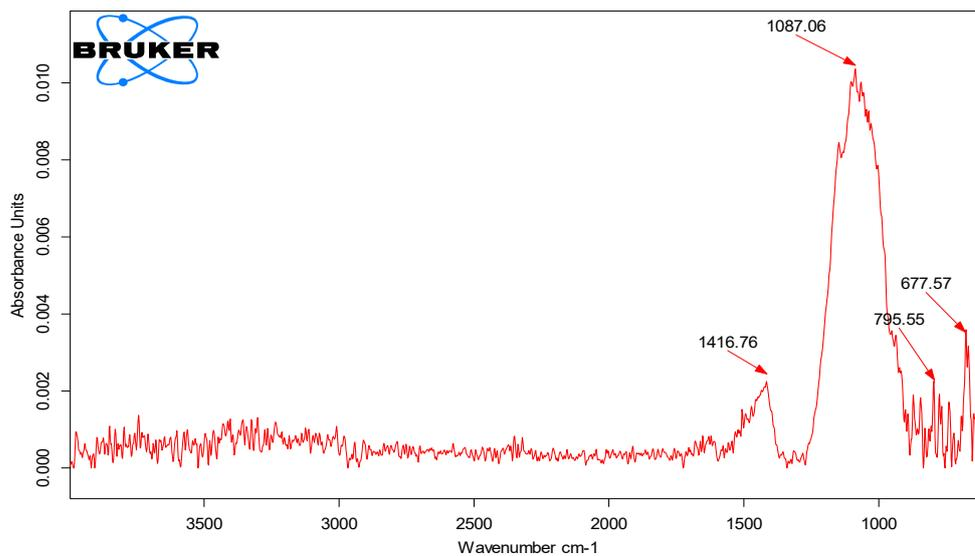
Fig. 2. IR spectrum of sulfur cake.
