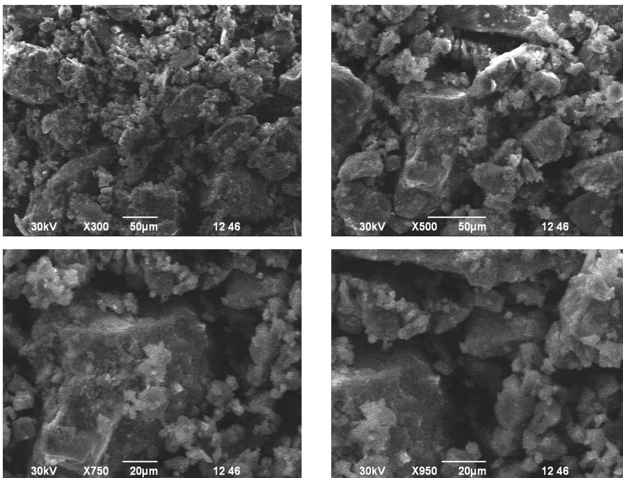
Fig. 3. Electron microscopic images of sulfur cake.
