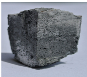
Fig. 5. Macrostructure of the gradient material produced as a part of the multilayered system combustion products.
