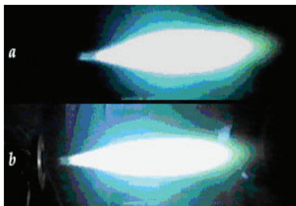
Fig. 6. Hydrogen flame in a supersonic air jet. M_2 = 2.2 ; M_1 = 1 . a: within input of hydrogen only; b: with input of hydrogen to the injector + H_2O_2 to the prechamber.
