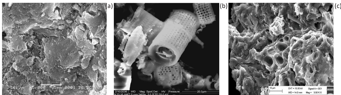
Fig. 8. SEM images of bentonite [119] (a), diatomite [120] (b), and activated carbon [121] (c). Reproduced from Ref. [119–121]. Licensed under a Creative Commons Attribution (CC BY) license.
