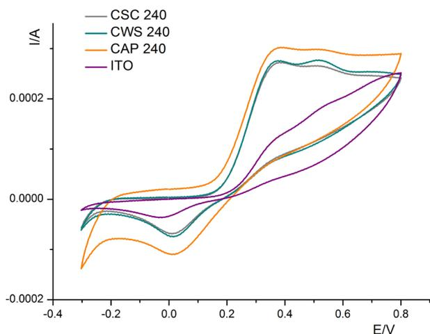
Fig. 6. Cyclic voltammograms of dopamine on the test electrodes obtained by hydrothermal carbonization.
