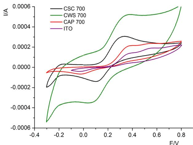
Fig. 5. Cyclic voltammograms of dopamine on the test electrodes obtained by thermal carbonization.
