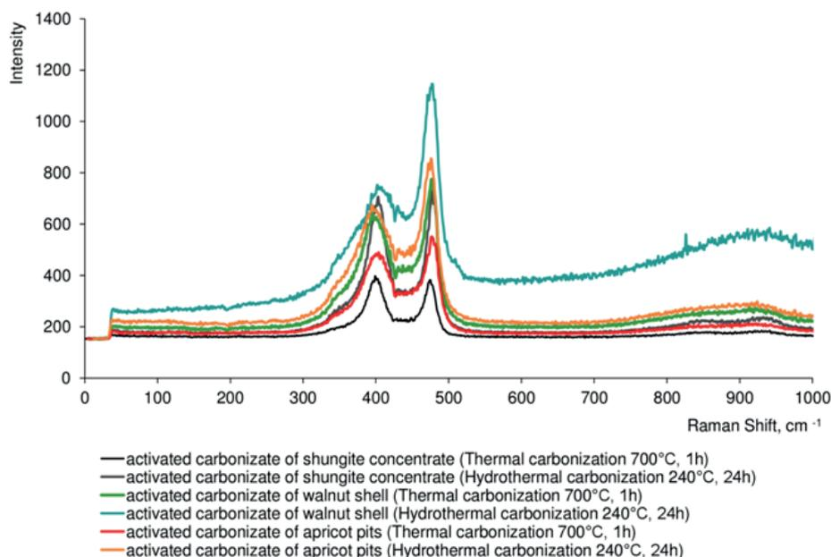
Fig. 2. Raman spectra of carbon containing electrode materials.
