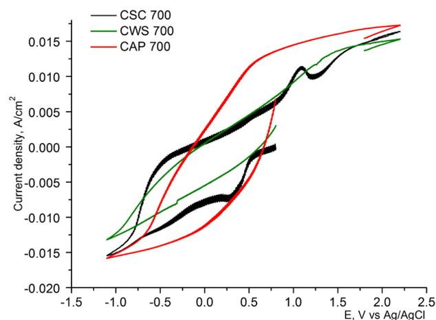
Fig. 4. CVA-curves of the test electrodes obtained by thermal carbonization.
