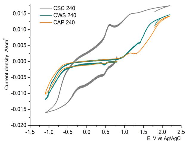
Fig. 3. CVA-curves on the test electrodes obtained by hydrothermal carbonization.
